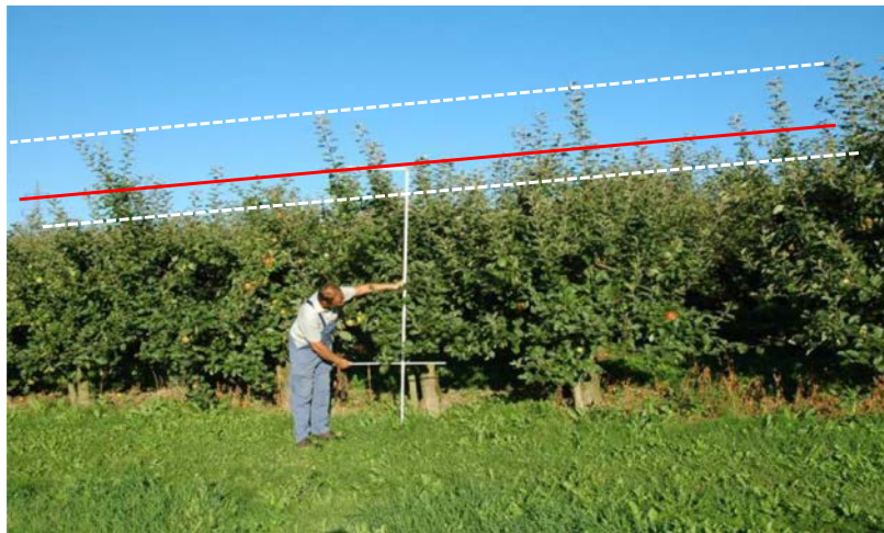
Fig. A13 Measurement of the treated canopy/crown/foilage height. The red line illustrates the measurement of the upper limit.
