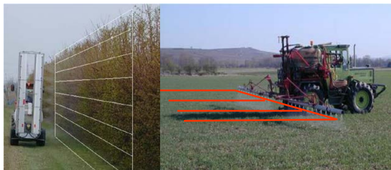
Fig. A1 Treated area is the oversprayed plane between working nozzles and targets.
